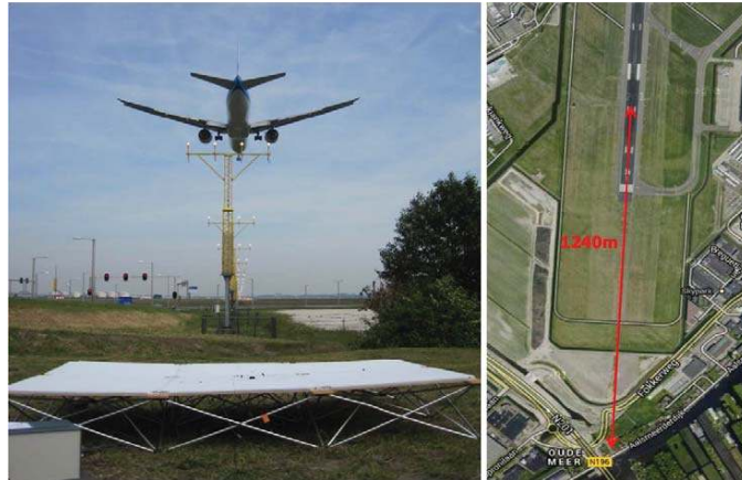
Fig. 8: Experimental set-up located 1,240 m to the South of the threshold of the Aalsmeerbaan (36R) Schiphol airport runway.
