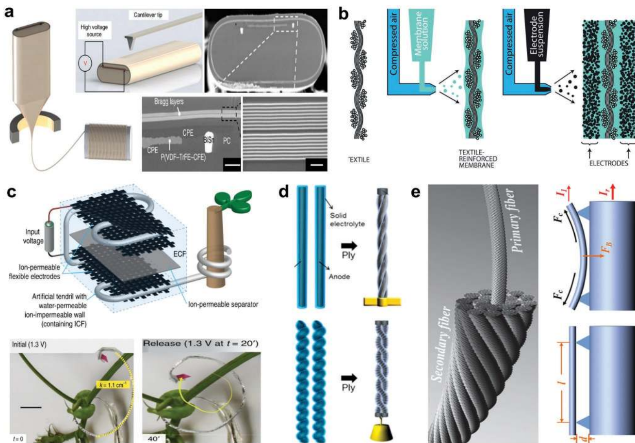
Figure 3. Electric actuated fibers/yarns. a) The thermally drawn fiber with piezoelectric PVDF. Reproduced under the terms of the CC-BY Creative Commons Attribution 4.0 International License ( http://creativecommons.org/licenses/by/4.0/ ). [68] Copyright 2017, The Authors, published by Springer Nature. b) An ionic and capacitive laminate actuator. Reproduced with permission. [73] Copyright 2017, Elsevier. c) A tendril like osmosis actuator that reversibly changed stiffness and performed hooking/anchoring. Reproduced under the terms of the CC-BY Creative Commons Attribution 4.0 International License ( http://creativecommons.org/licenses/by/4.0/ ). [79] Copyright 2019, The Authors, published by Springer Nature. d) All-solid-state actuator consisting of twisted CNTs fiber that infiltrated with solid electrolyte. Reproduced with permission. [80] Copyright 201, American Chemical Society. e) Current-actuated hierarchical CNTs fiber. Reproduced with permission. [81] Copyright 2014, Wiley-VCH.
