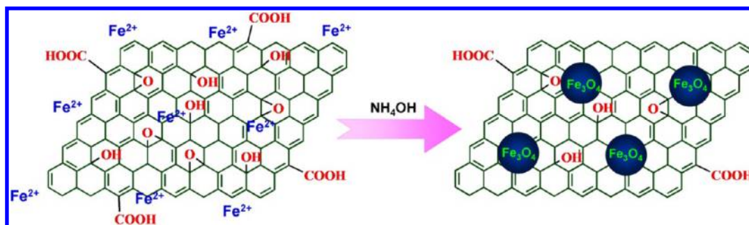
SCHEME 6. Synthetic Route to \text{Fe}_3\text{O}_4/\text{rGO} via Redox Reaction between GO and \text{Fe}^{2+} Ions. Adapted from reference 50 with permission. Copyright 2011, Royal Society of Chemistry.
