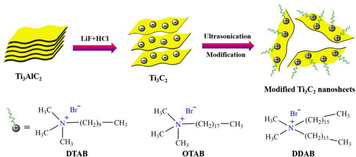
Scheme 1. Illustration for preparation of functionalized \text{Ti}_3\text{C}_2 (MXene) nanosheets. DTAB = decyltrimethylammonium bromide; OTAB = octadecyltrimethylammonium bromide; DDAB = dihexadecyldimethylammonium bromide.
