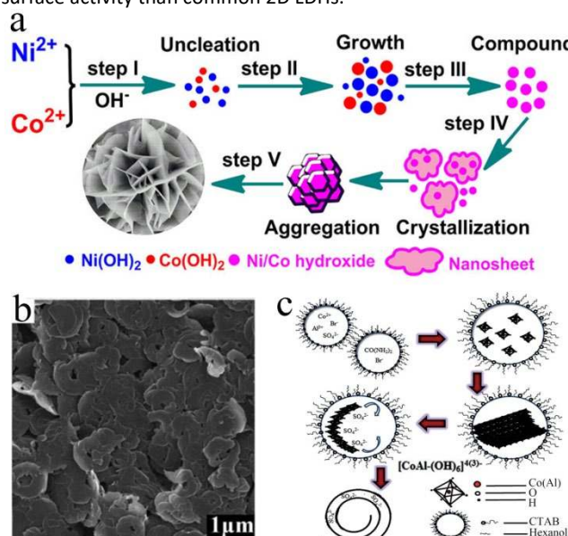
Figure 7. (a) Schematic illustration describing the synthetic procedures of the 3D NiCo-LDH microspheres, 229 Reproduced with permission from ref. 229 , Copyright 2016, American Chemical Society; (b) SEM image of MgAl-LDH nanorings, 233 Reproduced with permission from ref. 233 , Copyright 2011, The Royal Society of Chemistry; (c) schematic of the nucleation and structural
