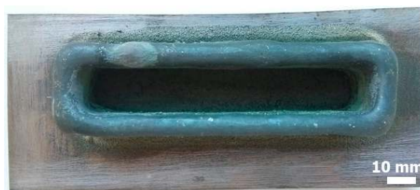
Figure 2. SS316L to Ni80-20 structure manufactured by 3DPMD, top view.
