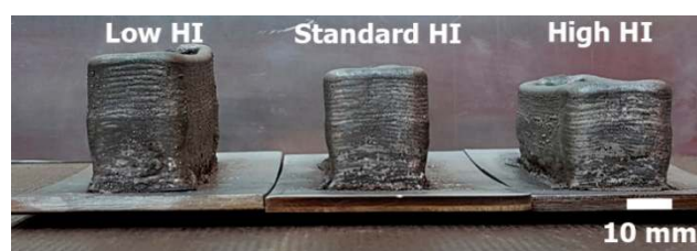
Figure 5. SS316L to Ni625 structures manufactured by 3DPMD.
