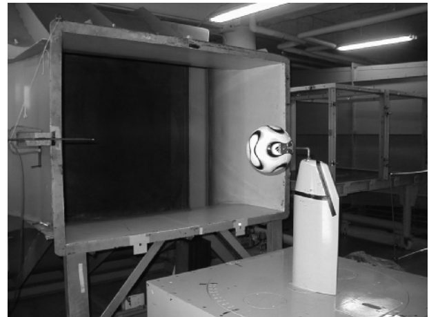
Figure 1 Wind tunnel experimental set-up for a non-rotating ball. The ball was supported at the back, with the tip mounted on a six-component wind tunnel balance.
