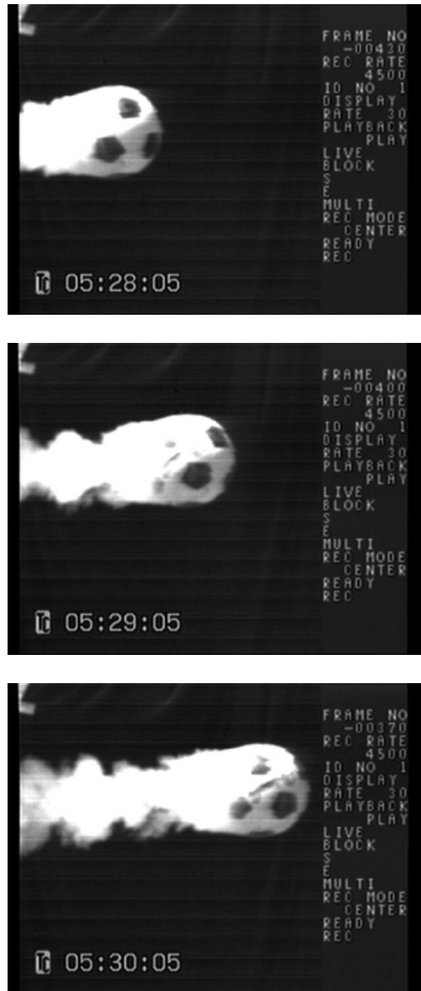
Figure 10 Series of side-view lateral images of a rotating ball in flight at 26 \text{ m s}^{-1} and 8 \text{ rev s}^{-1} ( S_p = 0.21 ). The time interval for each image was \sim 0.0067 \text{ s} . The separation point was \sim 120^\circ from the front stagnation point, and the vortex angle also reached \sim 120^\circ . The flow was from right to left.
