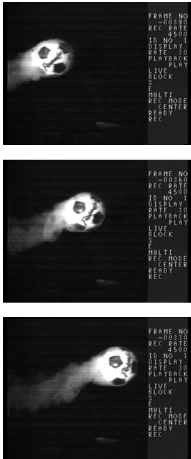
Figure 11 Series of top-view parietal images of a rotating ball in flight at 27 \text{ m s}^{-1} and 7 \text{ rev s}^{-1} ( S_p = 0.18 ). The time interval for each image was \sim 0.0067 \text{ s} . The vortex deviated, and the vortex angle reached \sim 128^\circ . The flow was from right to left.
