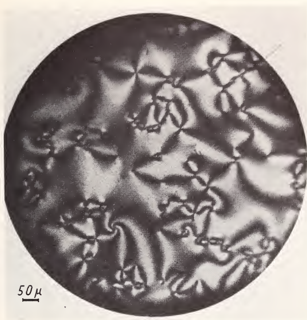
PLATE I. Nematic phase of azoxyphenetol; disclinations of strength 1 (four branches) and 1/2 (two branches) are seen end on, between crossed polars. (After G. Friedel.)
