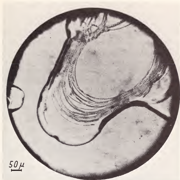
PLATE II. Terraced smectic droplet (after G. Friedel) of ethyl azoxybenzoate.
