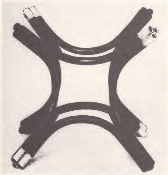
FIGURE 4. Three screw (wedge) disclinations of strength -1 . Courtesy of F. R. N. Nabarro.
