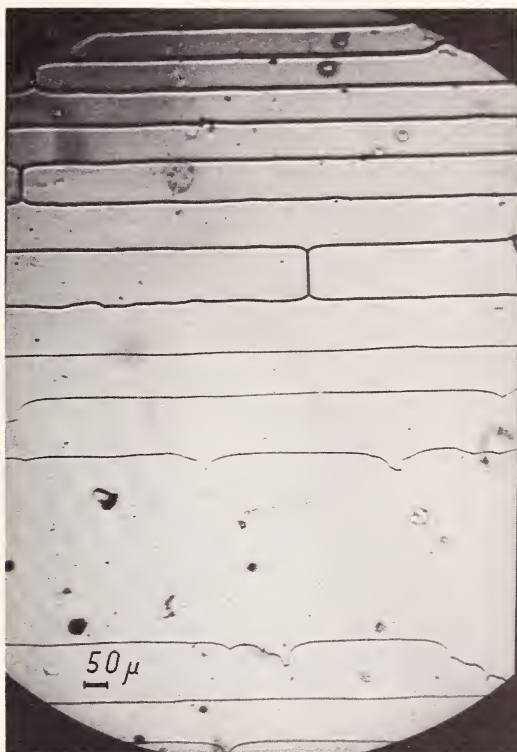
PLATE IV. High pitch cholesteric phase (dilute solution of a cholesterol ester in p . azoxy-anisole): observation of Grandjean-Cano walls. (Courtesy Orsay Liquid Crystal Group.)
