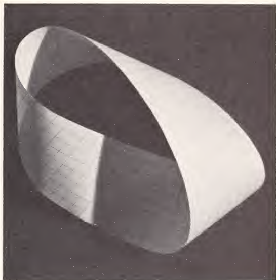
FIGURE 4. Global defect (Möbius strip) with components edge disclination ( \omega = \pi ), screw disclination ( \omega = 2\pi ) and edge dislocation.
