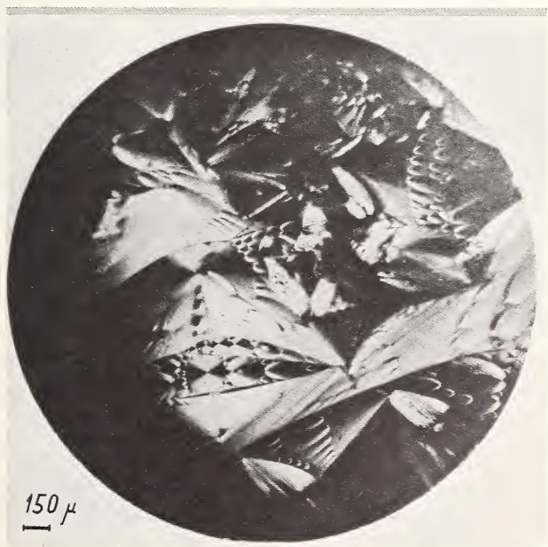
PLATE III. Cofocal domains in ethyl azoxybenzoate. Most of the ellipses are in the plane of the glass plate. Crossed polars.
