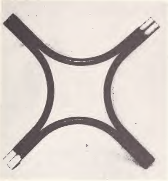
FIGURE 3. A screw (wedge) disclination of strength -1 . Courtesy of F. R. N. Nabarro.
