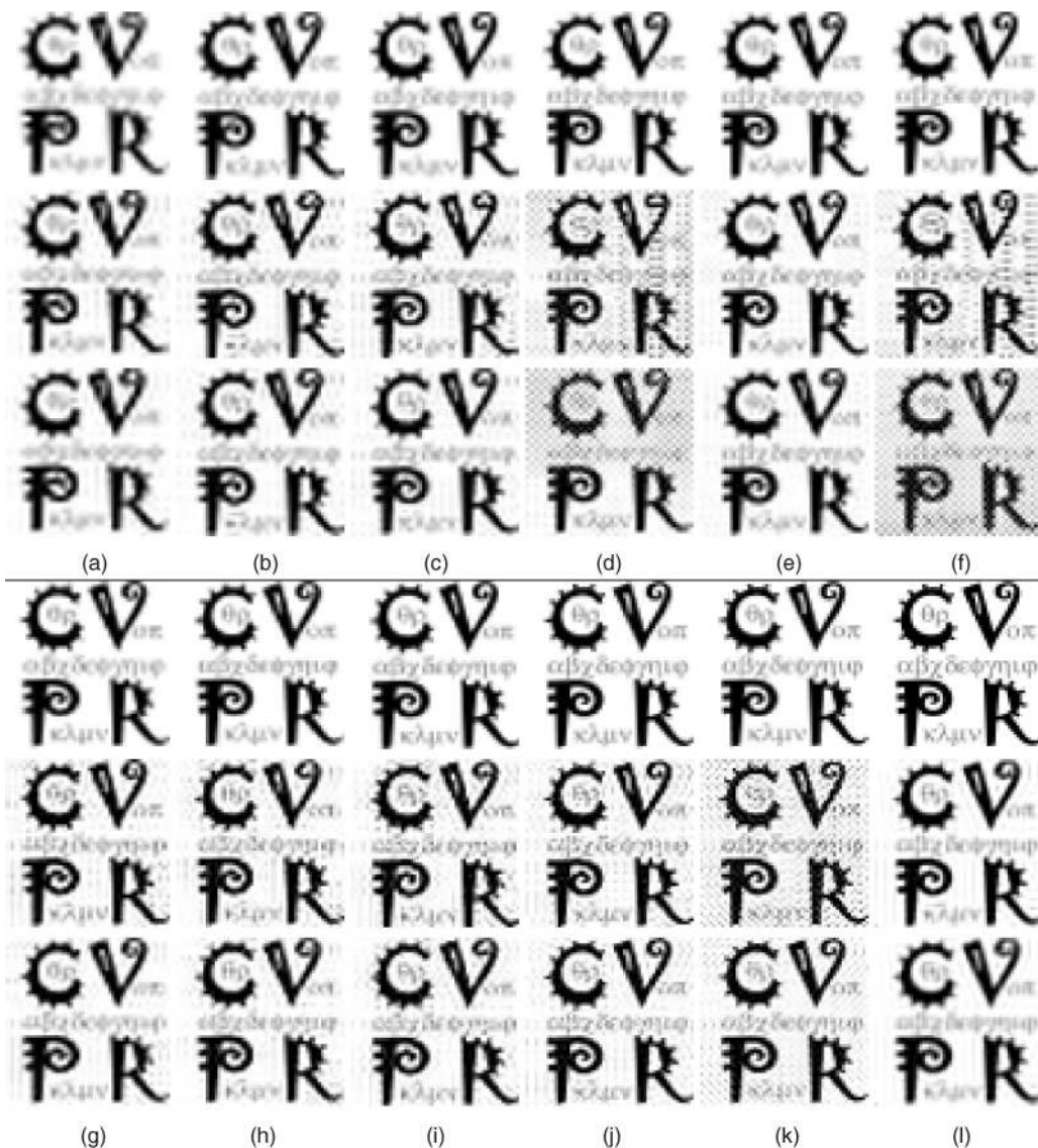
Fig. 9. The ground truth and superresolution results. The first and fourth rows are the ground truth images. The second and fifth rows are superresolution results using 36 LRIs. The third and sixth rows are superresolution results using the vertices sets only. They are all ML solutions except the second and third images of (e) and (l), which are MAP solutions with \lambda_s: 5 \times 10^{-14}, 5 \times 10^{-15}, 5 \times 10^{-2}, and 5 \times 10^{-2} , respectively. The criterion of choosing \lambda_s is that the resultant noise is approximately the same as that in the corresponding images in (c) or (j) in order to compare the resolution in a fair manner. Their corresponding ML solutions are random patterns and, hence, not shown here. The magnification factors are: (a) \mathcal{M} = 1.5 . (b) \mathcal{M} = 1.8 . (c) \mathcal{M} = 1.9 . (d) \mathcal{M} = 1.98 . (e) \mathcal{M} = 2.0 . (f) \mathcal{M} = 2.02 . (g) \mathcal{M} = 2.15 . (h) \mathcal{M} = 2.3 . (i) \mathcal{M} = 2.5 . (j) \mathcal{M} = 2.8 . (k) \mathcal{M} = 2.94 . (l) \mathcal{M} = 3.0 .
