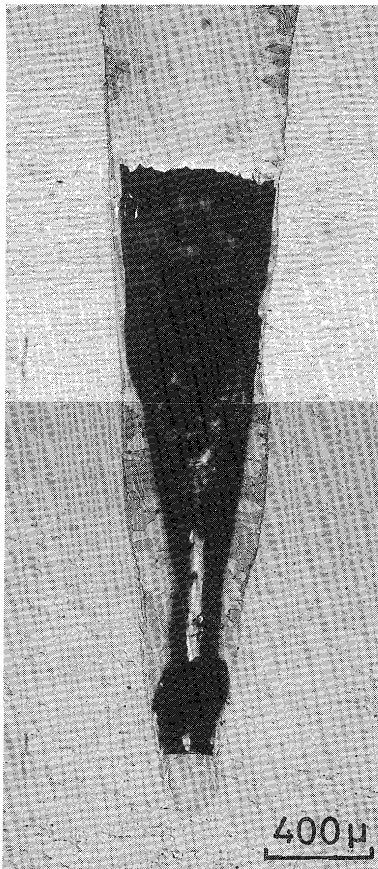
Photo. 1 Typical R-porosity (SUS 316)
