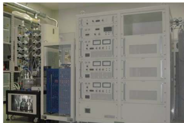
Fig. 15 A flow-type manufacturing system for syntheses of nanoparticles (co-work with Kurita Seisakusho).
