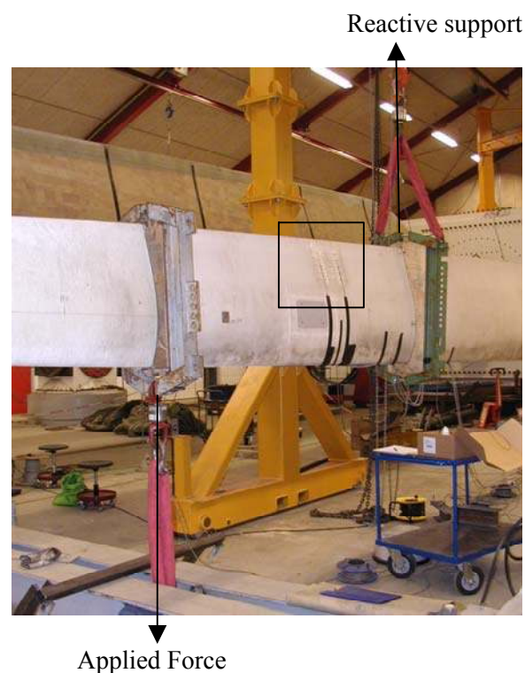
Figure 9. Test set-up, test-series 1. The framed area is the down-wind surface of the same area as shown in Figure 7.
