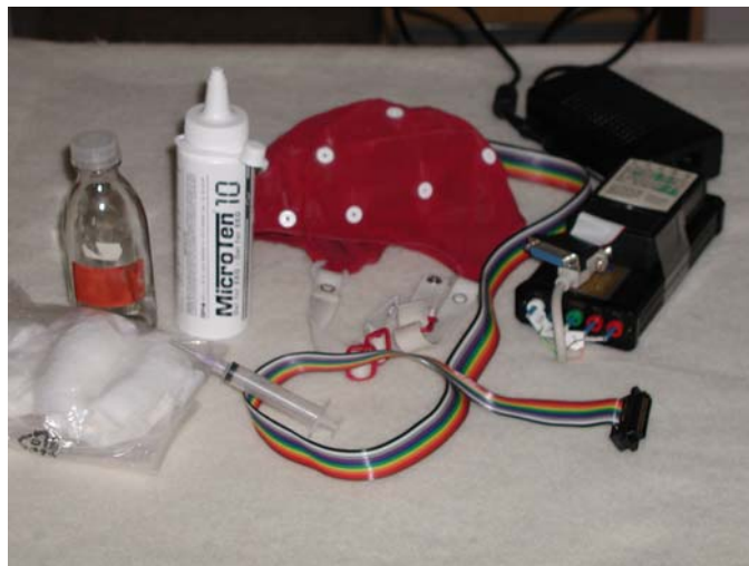
Figure 2. Equipment for EEG recording: amplifier unit, electrode cap, conductive jelly, injection, and aid for disinfection.
