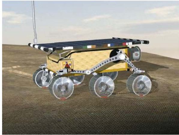
Fig. 1.16 A computer model of the Sojourner, produced with Vortex (image courtesy of CM Labs Simulations Inc.)
