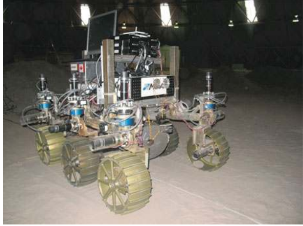
Fig. 1.15 Rover Chassis Prototype (RCP) undergoing tests at the University of Toronto Institute for Aerospace Studies (UTIAS) Mars Dome (courtesy of MDA Corporation, Brampton, ON)
