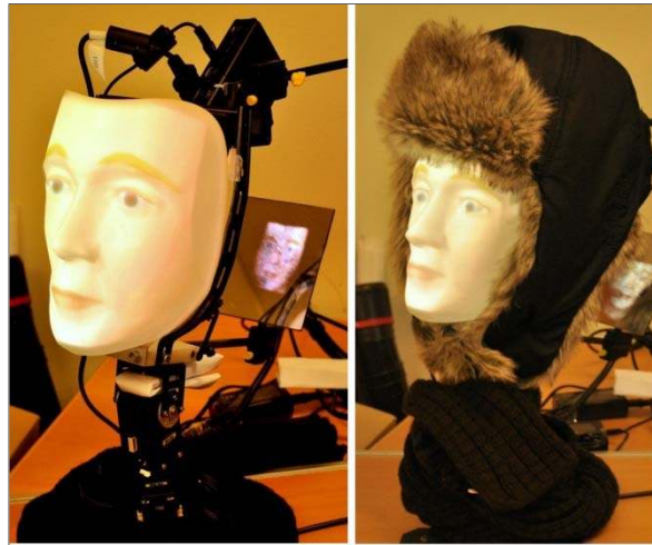
Fig. 9. Snapshots of Furhat with and without the head cover (the fur hat).
