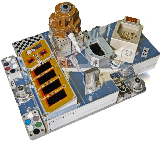
Fig. 3. Passive experiment samples on the front side of TB4.
