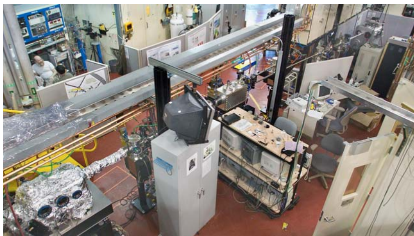
Figure 1. Beamline 11.0.2 at the ALS. The monochromator is foil-wrapped at the lower left. The line branches by means of a movable mirror and each branch has its own set of exit slits. The STXM branch is seen here, with the STXM enclosure to the upper right.
