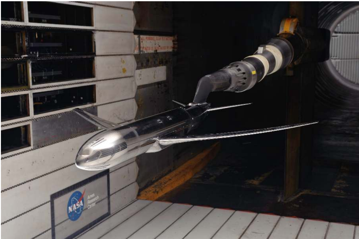
Figure 7. Photo of the Common Research Model in the Ames 11-ft Wind Tunnel.
