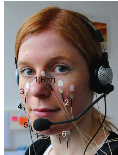
Fig. 1. Electrode positioning, black numbers indicate unipolar derivation with reference electrodes on mastoid portion of the temporal bone (except channel 1), white numbers indicate bipolar derivation.
