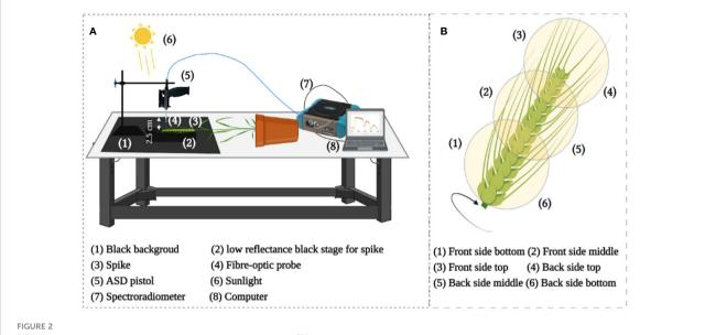
(A) Illustration of the setup for hyperspectral measurement, (B) Reflectance acquisition points from the whole individual spike.
