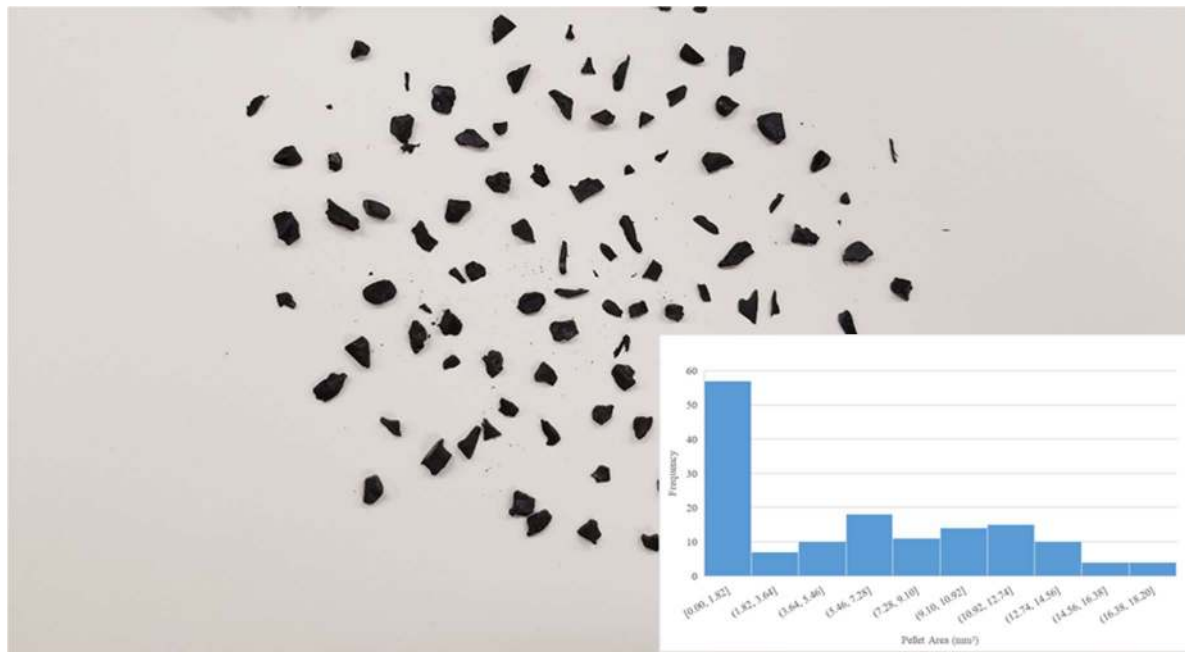
Figure 7. Recycled polypropylene (PP) flake size distribution.
