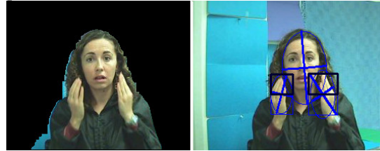
Fig. 3 Camshift tracking when hands are about to merge with the face. The darker rectangles represent the position of the fingers.
