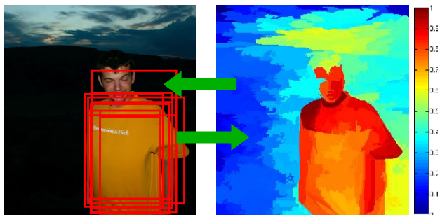
Figure 1. Mutual improvements between objectness and saliency. Left: Each red window indicates a possible object within it. (Note that we always draw the top 10 objectness windows for illustration.) Right: The estimated saliency map, where the color bar on the right shows the scales of saliency values.
