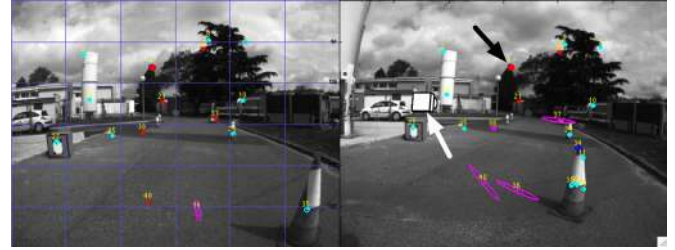
Fig. 12. Snapshots of master and slave sequences in cooperative SLAM. Faraway landmarks (e.g., black arrowed), still initialized as rays (red), are the ones fixing the orientation. Nearby landmarks, usually as Euclidean points (blue), maintain the metric. A virtual model of the master camera is visible from the slave camera (white arrowed). See cooperativeSLAM.mov .
