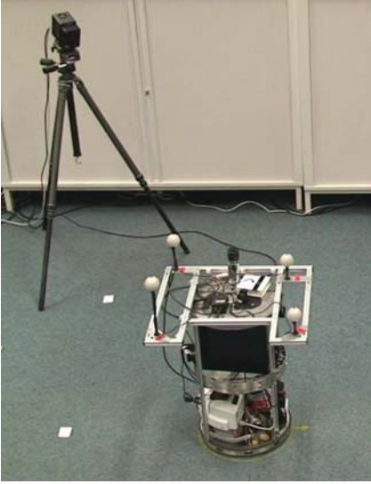
Fig. 1. Service robot platform Robotino with omni-directional drive used for evaluation. On top there are camera and markers required for the reference positioning system Dtrack.
