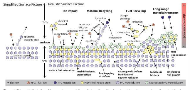
**Figure 1.** Schematic illustration of the complex, synergistic, and inherently multiscale surface interactions occurring at the material surface in a realistic magnetic fusion plasma environment. H, hydrogen; D, deuterium; T, tritium; PFC, plasma facing component; γ, gamma ray.
