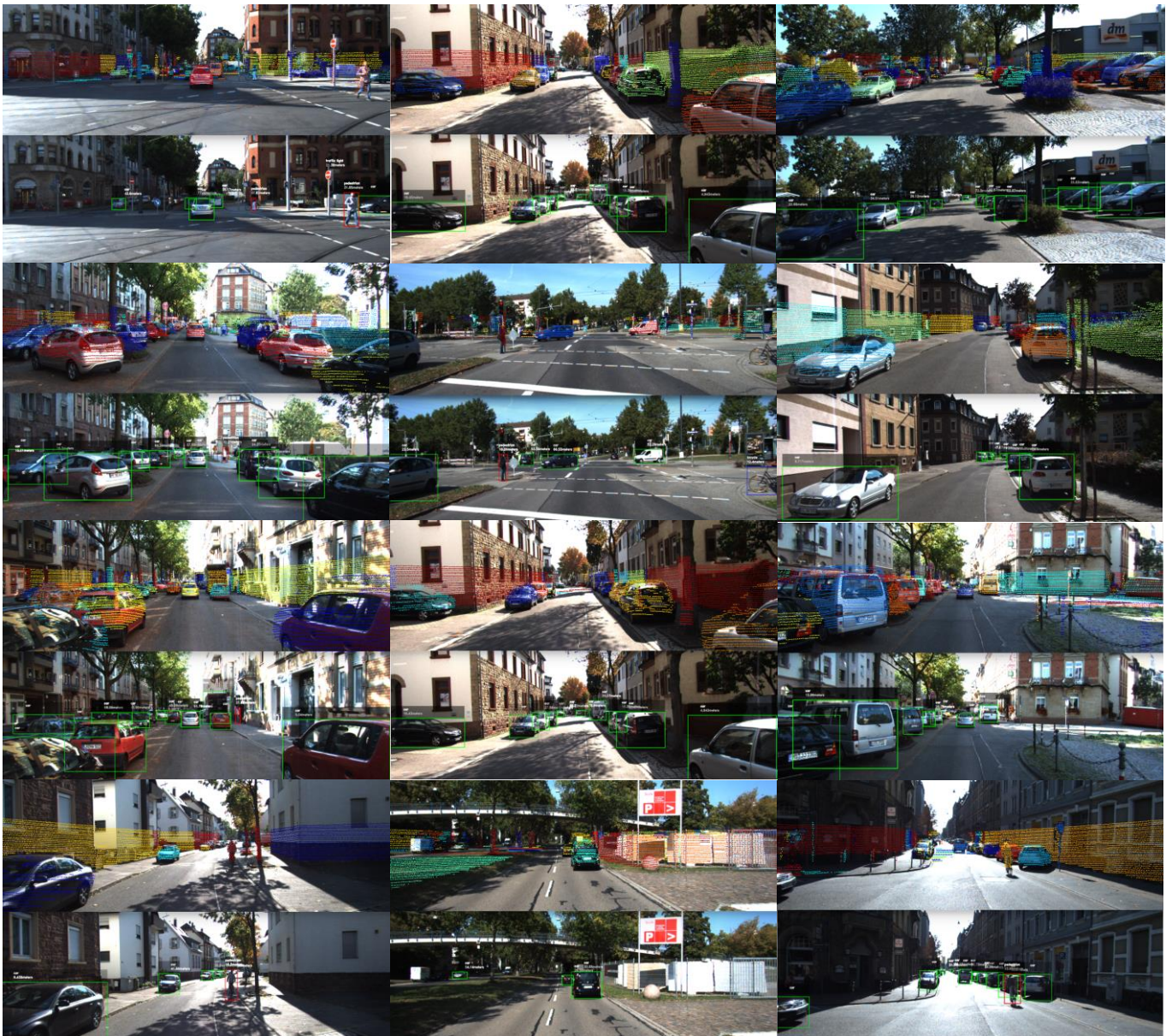
Fig. 11. Examples of object detection results using our proposed method on the KITTI benchmark dataset [12], including Pedestrians and Cars at various difficulty levels.
