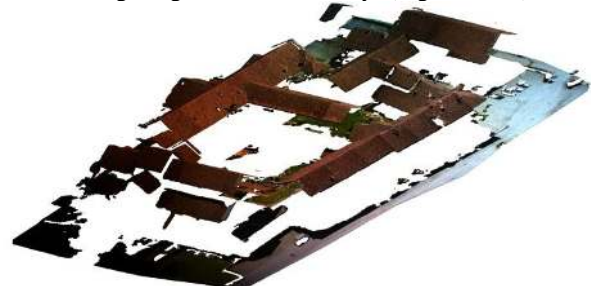
Figure 19. Point cloud extracted using MicMac software
