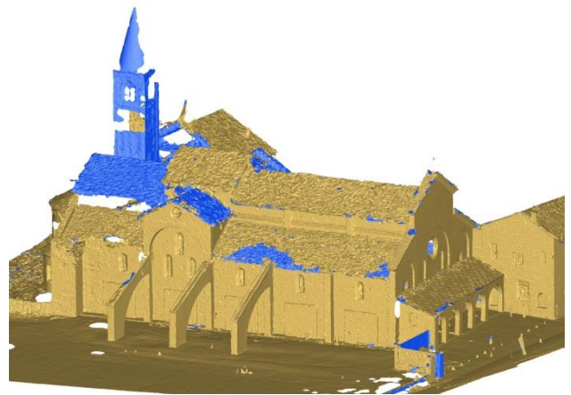
Figure 18. 3DModel processed with regular sampling method (distance between points of 0.2 m) from data fusion.
