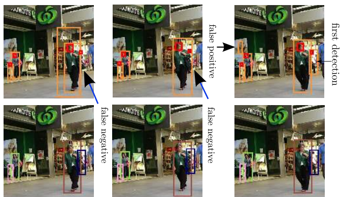
Figure 1. MOT16-09 sequence (from left to right: frame 10,12,15). Top row: Body detections (orange) and head detections (red). The body detector misses the person depicted by the arrow until frame 15. Bottom row: The result of our tracker. The false positive is removed as it does not have a corresponding head detection. The tracker recovers the heavily occluded pedestrian due to the presence of head detections.
