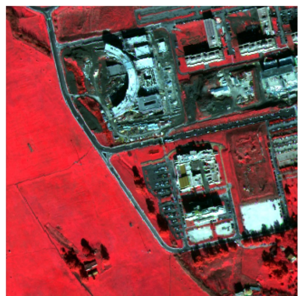
Figure 5 False color composite obtained combining NIR1, RED and GREEN bands of the original WorldView-2 image.
