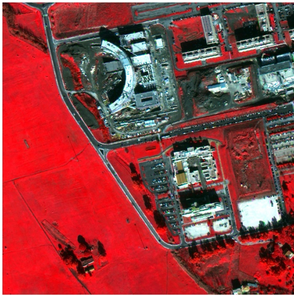
Figure 6 False color composite obtained combining NIR1, RED and GREEN bands of the fused WorldView-2 image.
