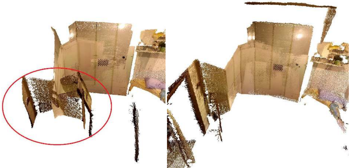
Figure 6. Partial 3D reconstruction of a poorly textured room using visual measurements only (left) and fusing inertial and visual measurements (right).
