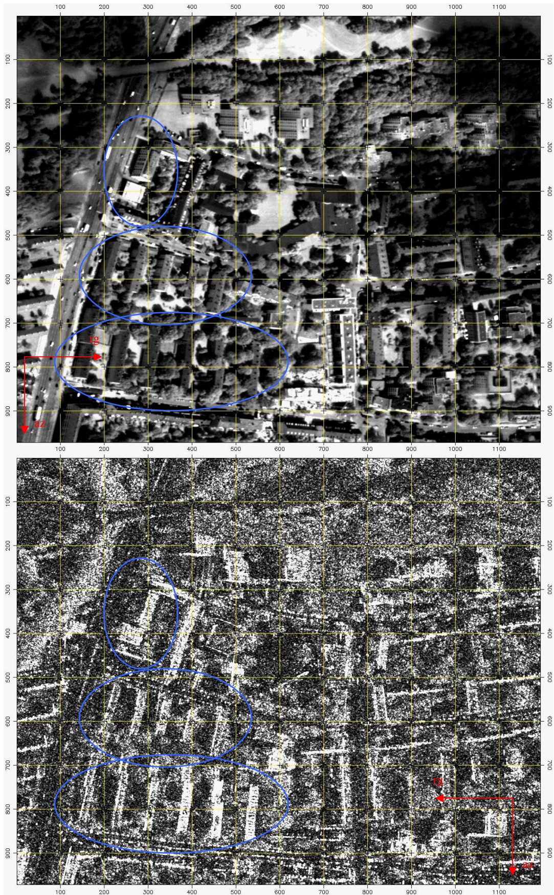
Figure 7. Part of Munich city acquired by VW-1 (upper image) and TS-X (lower image) using the proposed satellite formation. Yellow grid lines are for better orientation between two images. Red arrows show flight (az) and look (rg) directions.
