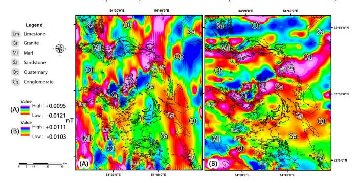
**Figure 9.** Horizontal derivative map for the study area. (**A**) horizontal derivative filter in the direction of 45-degree azimuth; (**B**) horizontal derivative filter in the direction of 135-degree azimuth.
