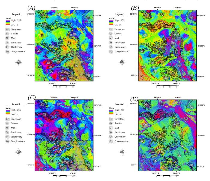
**Figure 4.** Spatial distribution of iron oxide/hydroxides and hydroxyl-bearing (Al-OH) alteration and carbonates in the study area as pseudo-color ramp. (**A**) 4/2 band ratio of Sentinel-2; (**B**) 1/3 band ratio of Landsat-7; (**C**) 11/12 band ratio of Sentinel-2; (**D**) 5/7 band ratio of Landsat-7.
