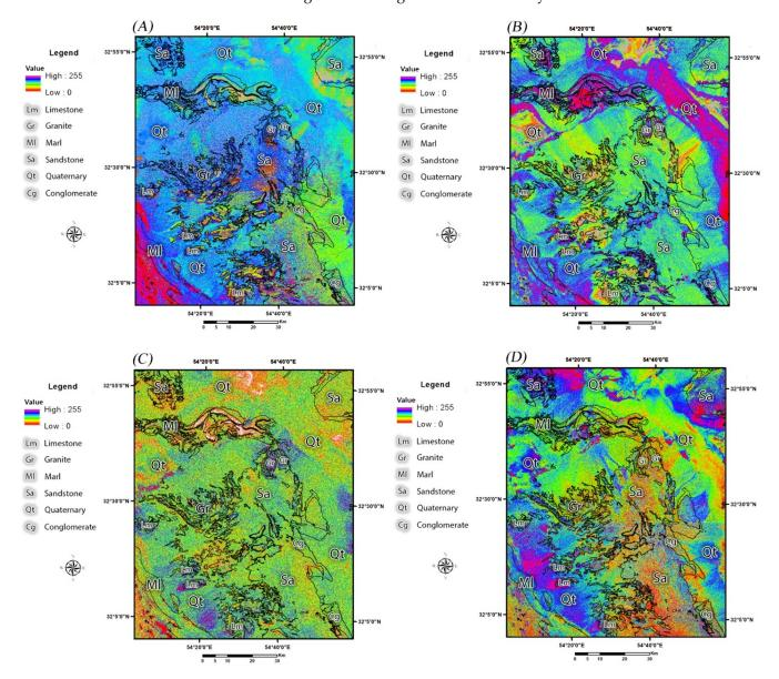
**Figure 6.** Spatial distribution of iron oxide/hydroxides and hydroxyl-bearing (Al-OH) alteration and carbonates in the study area as pseudo-color ramp. (**A**) LS-Fit residual band 4 of Sentinel-2; (**B**) LS-Fit residual band 12 of Sentinel-2; (**C**) LS-Fit residual band 3 of Landsat-7; (**D**) LS-Fit residual band 7 of Landsat-7.
