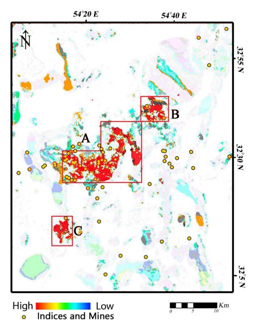
**Figure 10.** Potential map for the study area derived from the fuzzy logic model. High potential zones (**A–C**) are delimited by red lines. The yellow dots are the locations of mineralization that were documented and visited in the field survey.
