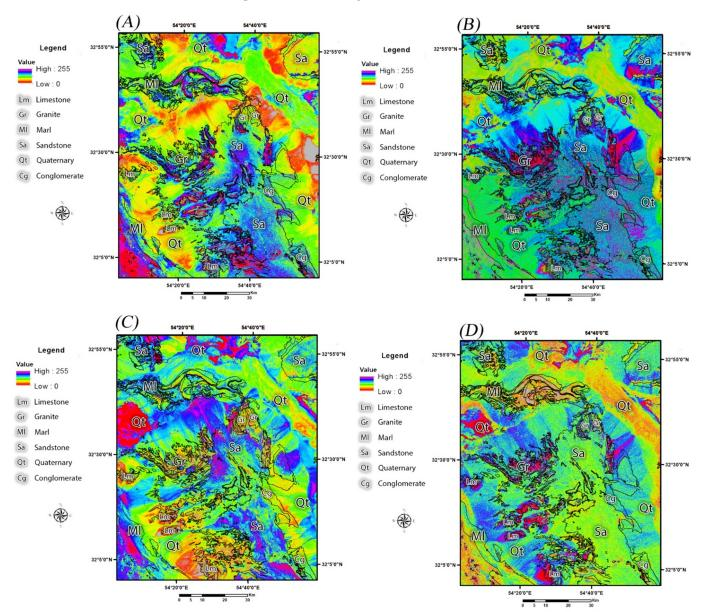
**Figure 5.** Spatial distribution of iron oxide/hydroxides and hydroxyl-bearing (Al-OH) alteration and carbonates in the study area as pseudo-color ramp. (**A**) PCA2 image of Sentinel-2; (**B**) PCA4 image of Sentinel-2; (**C**) PCA3 image of Landsat-7; (**D**) PCA4 image of Landsat-7.
