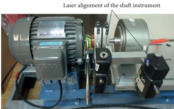
FIGURE 6: Setup of laser alignment of the shaft.
