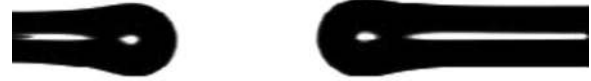
Fig. 2. Side views of the splicing joint on the screen of the FSU-975 splicer using the program set for conventional SMFs when HC-1550-02 is spliced to SMF-28.
