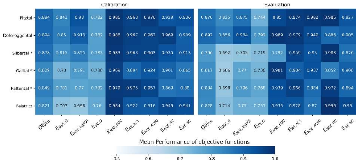
Figure 3. Mean model performance of the best 300 parameter sets for the calibration and evaluation periods. Obj tot shows the overall model fit. Table 4 gives a description of the objective functions. The asterisk (*) indicates the catchments that use 8 years of evaluation instead of 10.
