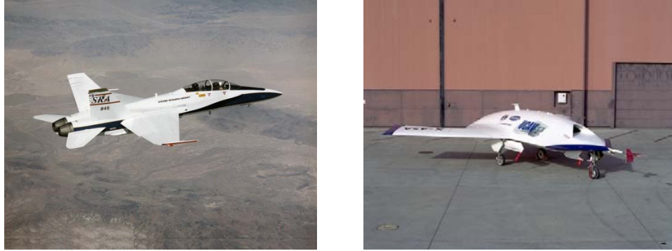
Figure 1: The F-18 aircraft, one of the first production military fighters to use “fly-by-wire” technology, and the X-45 (UCAV) unmanned aerial vehicle. Photographs courtesy of NASA Dryden Flight Research Center.
