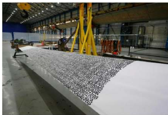
Fig. 16. Illustration of a fabric blade prototype tested in the Offshore Renewable Energy Catapult laboratories. Courtesy of ACT Blade Ltd.
