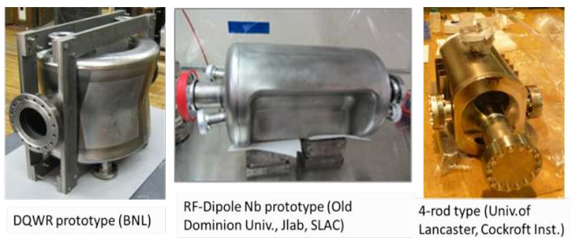
Fig. 17. The three types of compact crab cavities under development for HL-LHC.
