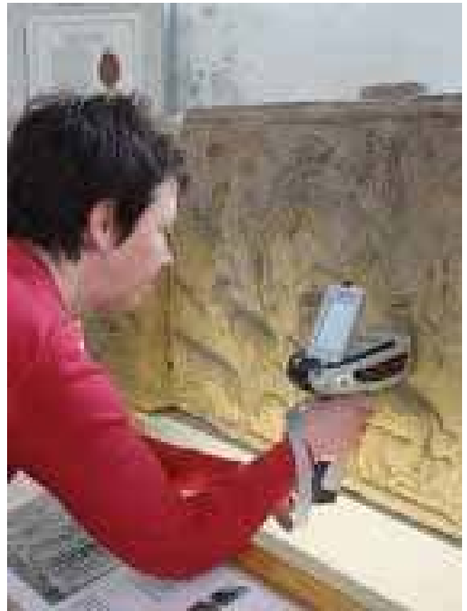
Figure 79: Historic Scotland Conservation Group using X-ray fluorescence to try to identify a white coating on the St Andrews Sarcophagus. © Sally Foster
