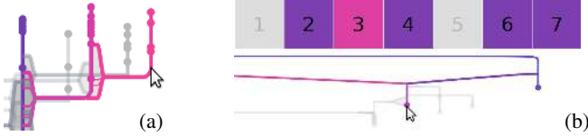
Figure 8: (a) Branch highlighting. The selected branch and all ancestors are highlighted with all connected saddles. (b) Member highlighting. Each member containing an edge in the selected bundle is highlighted in the associated color.
