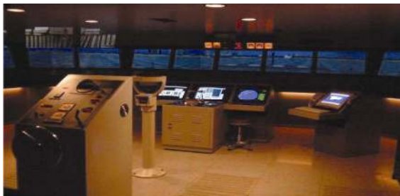
Fig. 11. Ship handling simulator SA PILOTSHIP 2000.
