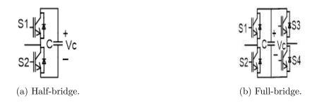
Figure 3.12: Half-bridge and full-bridge configuration of submodule.
