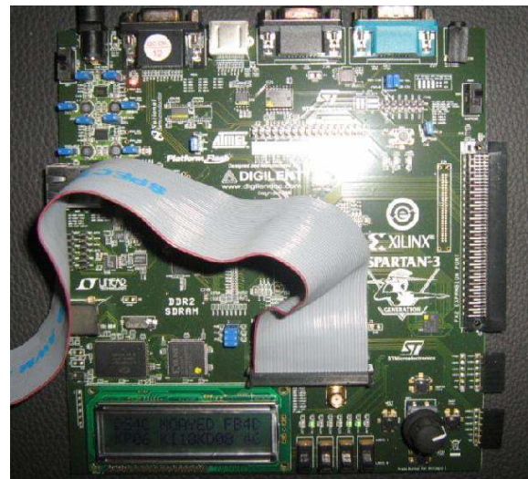
Figure 23. FPGA card with LCD and controlling keys.
