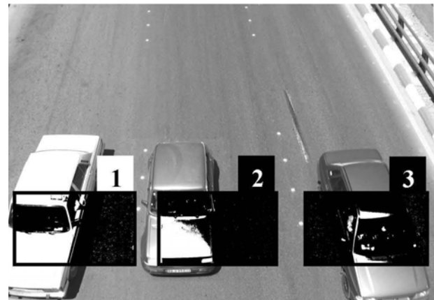
Fig. 3 Result of vehicle detection using classic running average and classic background subtraction.
