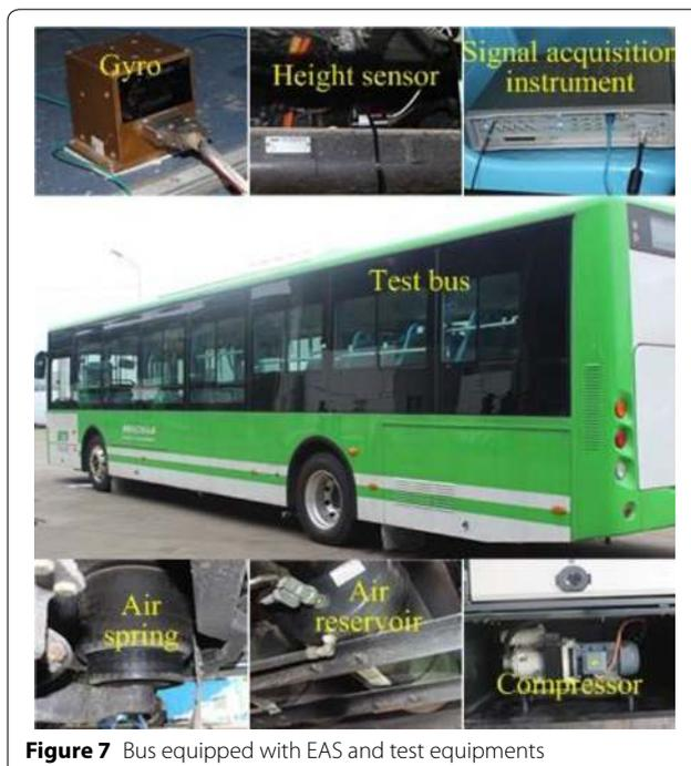
**Figure 7** Bus equipped with EAS and test equipments
