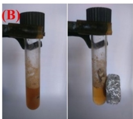
Figure 7. (A) Magnetization curves of (a) \gamma\text{-Fe}_2\text{O}_3 and (b) \gamma\text{-Fe}_2\text{O}_3\text{@SiO}_2\text{-EC-Zn}^{\text{II}} (V), (B) Catalyst ability for effective recovery at the end of reactions by an external magnetic field.
