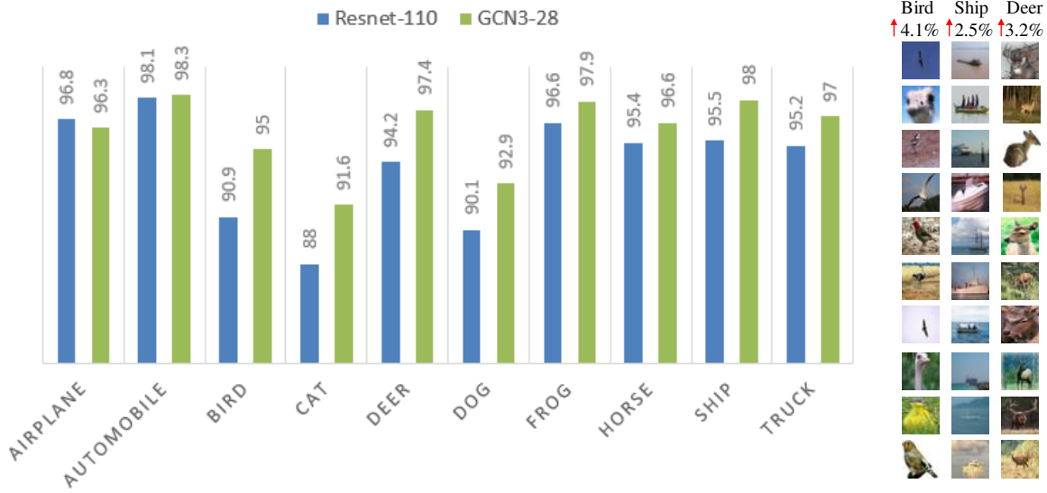
Fig. 7. Recognition results of different categories on CIFAR10. Compared with ResNet-110, GCNs perform significantly better on the categories with large scale variations.
