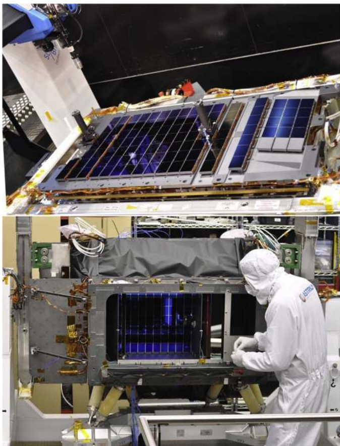
Fig. 5. Top: Gaia focal plane during assembly. The 14 SkyMapper CCDs are the first two full vertical strips on the left of the SiC structure and the 12 RVS CCDs on the right (the fifth row of white rectangles are not CCDs but are used in thermal control). Bottom: integrated focal plane showing the baffles and radiator (extended structure on each side). Again, the RVS CCDs are on the right.
