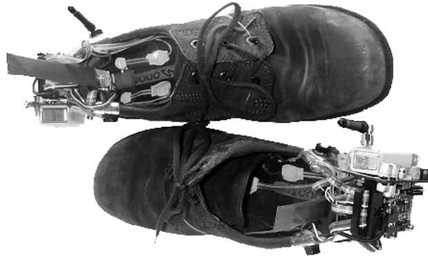
Figure IV. GaitShoe hardware mounted on shoes
